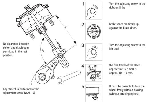
Special instructions apply for automatic slack adjusters (see adjustment procedure on the following pages).
